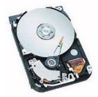
**Seagate 200GB HD** The Barracuda 7200.7 200GB hard disc drive delivers 7,200 RPM access speed and an Ultra ATA-100 interface for high-performance desktop applications.
